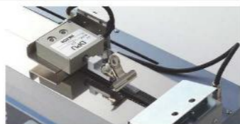
Peel test of embossed carrier tape
