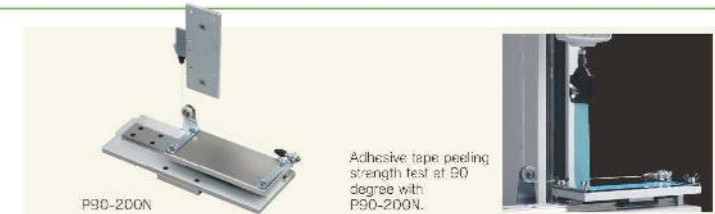
Adhesive tape peeling strength test at 90 degree with P90-200N. We provide a film cutter (P44). With the cutter, you can cut film in constant-width. We also provide a rubber roller according to JIS (See P44 for further information).
