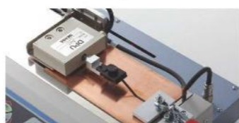
Peel test of copper foil
