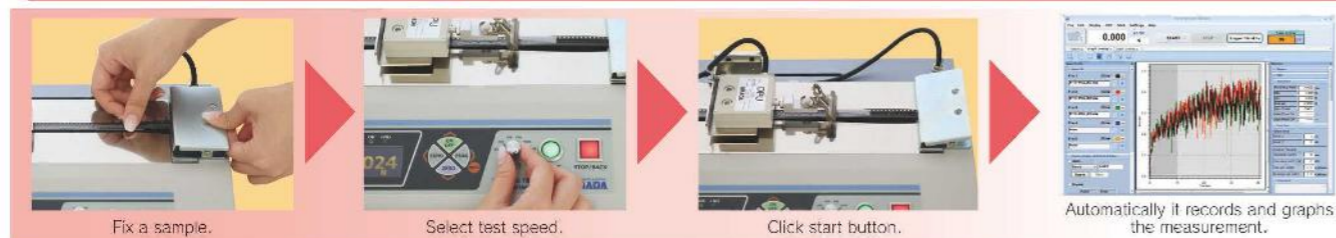
Peel test of copper foil
