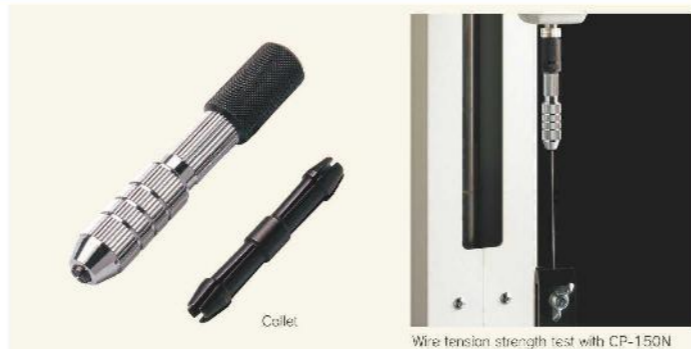
Wire tension strength test with CP-150N
